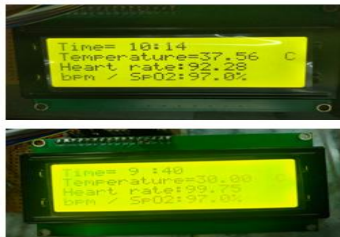
Fig. 3 - Prototype display showing the results of the vital signs.
