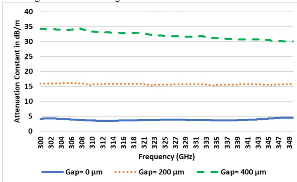
Fig. 6- Effect of Gap on the Attenuation Constant
