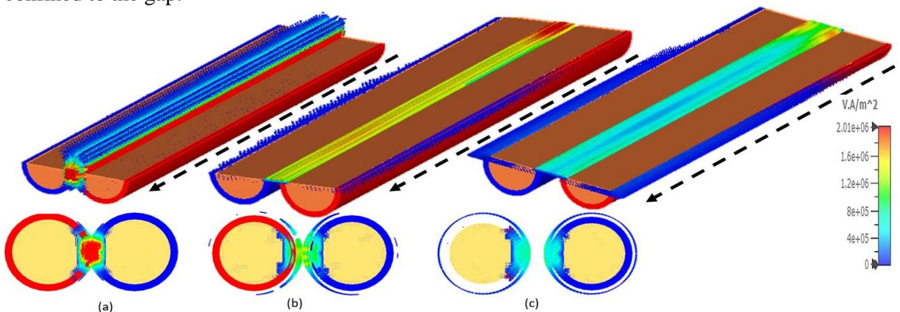
**Fig. 8- Effect of Gap on the Power Flow (a) 0  $\mu\text{m}$  gap (b) 200  $\mu\text{m}$  gap (c) 400  $\mu\text{m}$  gap**
