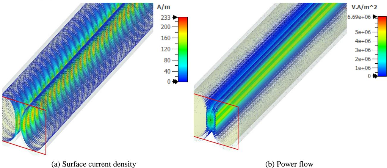
**Fig. 4- 3D simulation Analysis for Current Density and Power Flow**
