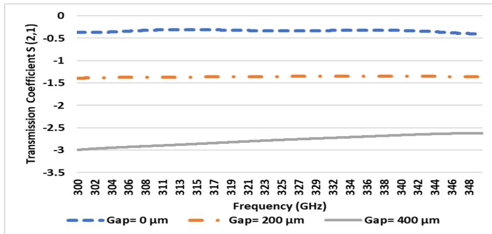
Fig. 5- Effect of Gap on the Transmission Coefficient S (2,1)
