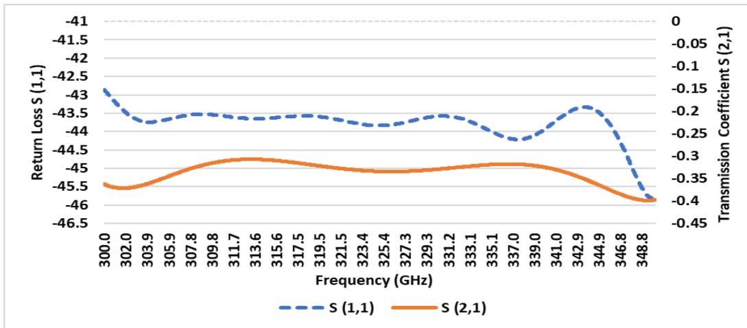
Fig. 2- Return Loss  $S(1,1)$  and Transmission Coefficient  $S(2,1)$  for two-wire power line
