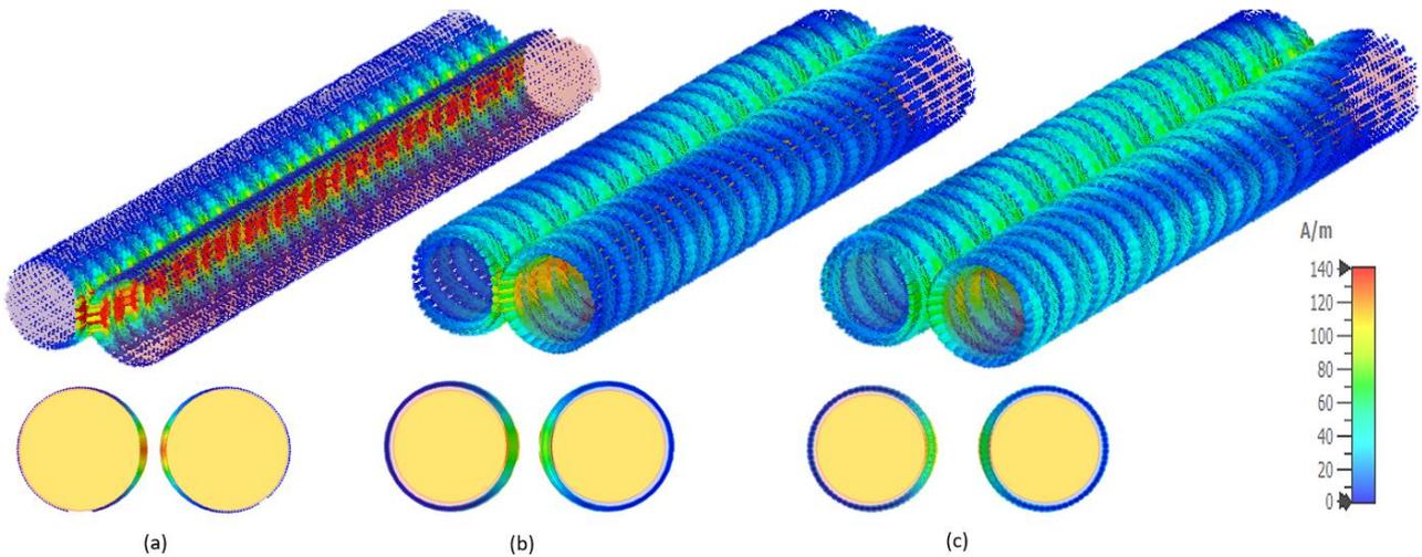
**Fig. 7- The effect of the Gap on the Surface Current Density (a) 0  $\mu\text{m}$  gap (b) 200  $\mu\text{m}$  gap (c) 400  $\mu\text{m}$  gap**
