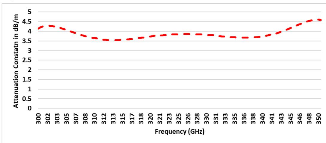
Fig. 3- Attenuation Constant in dB/m for two-wire power line
