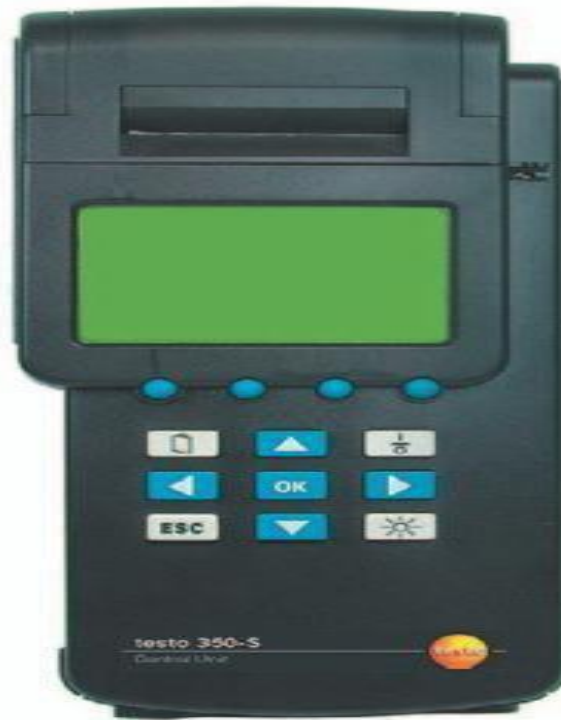
Fig. 3 - Gas analyzer control unit
