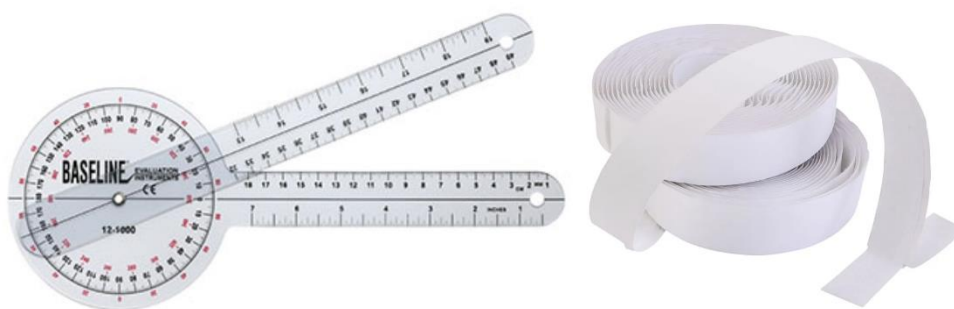
Fig. 7 - Anthropometric Equipment used for measuring angle of joints
