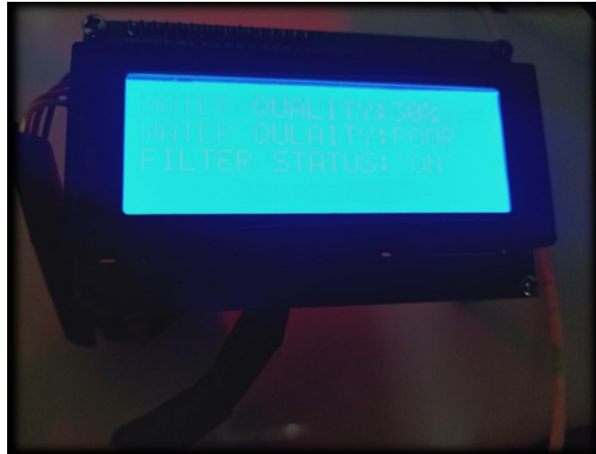
Fig. 14 – LCD showing water quality in percentage
