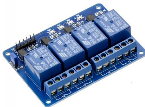
Fig 11 – Four Channel Relay
