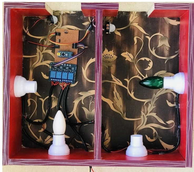
Fig. 8 – Automated Energy Saving System
