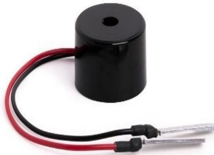
Fig. 4 -Buzzer used in Electronic Voting Machine
